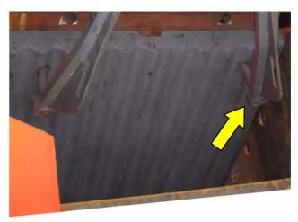
7. This is WRONG. The swing jaw must have no clearance with the jaw face. Adjust the swing jaw plate with the crane.
