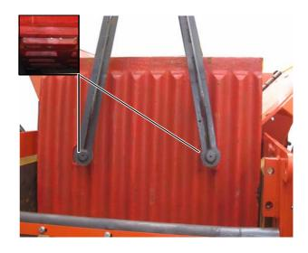
12. The hydraulic ram release with the fixed jaw plate removed, looks as shown.
