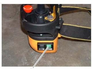
8. If necessary engine Revs Per Minute (RPM) can be adjusted up (faster) or down (slower) to aid tracking using buttons as shown.
