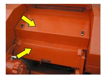
2. Install the inlet chute cover (1).
