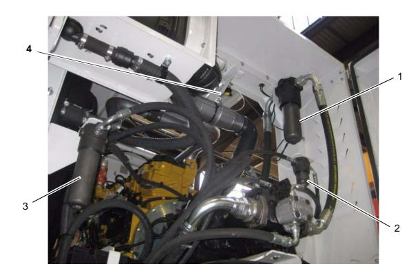
Figure 6-4: Engine Compartment - Filter element locations (for replacement)
