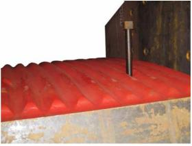
3. Attach the lifting hooks to a minimum of a 5 tonne (Metric) or 6 ton (US) crane.
