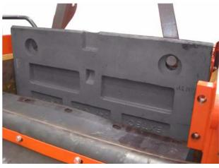
5. The jaw plate recesses will audibly drop onto the location point.
