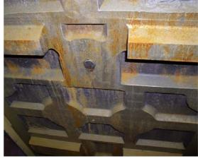
7. Use the crane and lower the plate into position, SLOWLY into the crusher box. Make sure the a clearance of 10mm to 15mm is between both sides.
