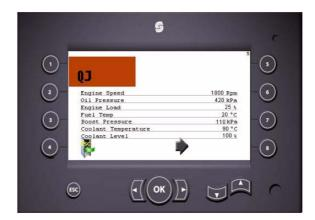
To access screen 2 of the engine parameters, press the right arrow button.
