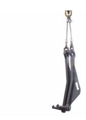
4. Install the Lifting hooks into the lifting eyes correctly. Tighten the chain/ropes with the crane.
