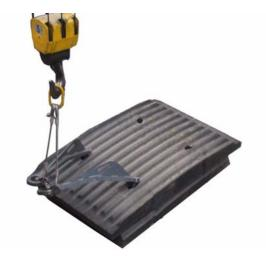
Make sure the lifting tool is installed correctly in the hole. Lift the fixed jaw plate with a minimum of a 5 tonne (Metric) or 6 ton (US) crane.
