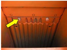
13. NOTE: Remove the wedge bolts as shown; pull out the wedge up the bolt. Remove the wedges and the bolt.
