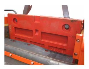
18. When the jaw plate is away from the machine move it down.
