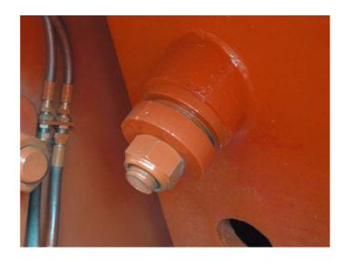
12. Use a crane with a strap/chain (lifting eye) to lift and hold the wear plate into position. Install and tighten the bolts with the nuts and washers.
