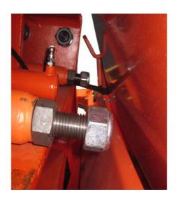
12. Adjust the fixed jaw plate as necessary and make sure it is centred.
