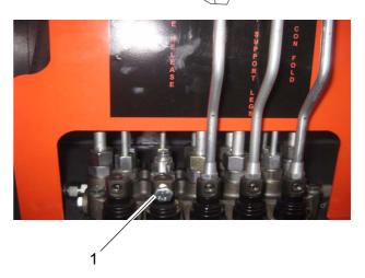
17. Loosen and remove the spare lever. Install and tighten the bolt with the nut (1).
